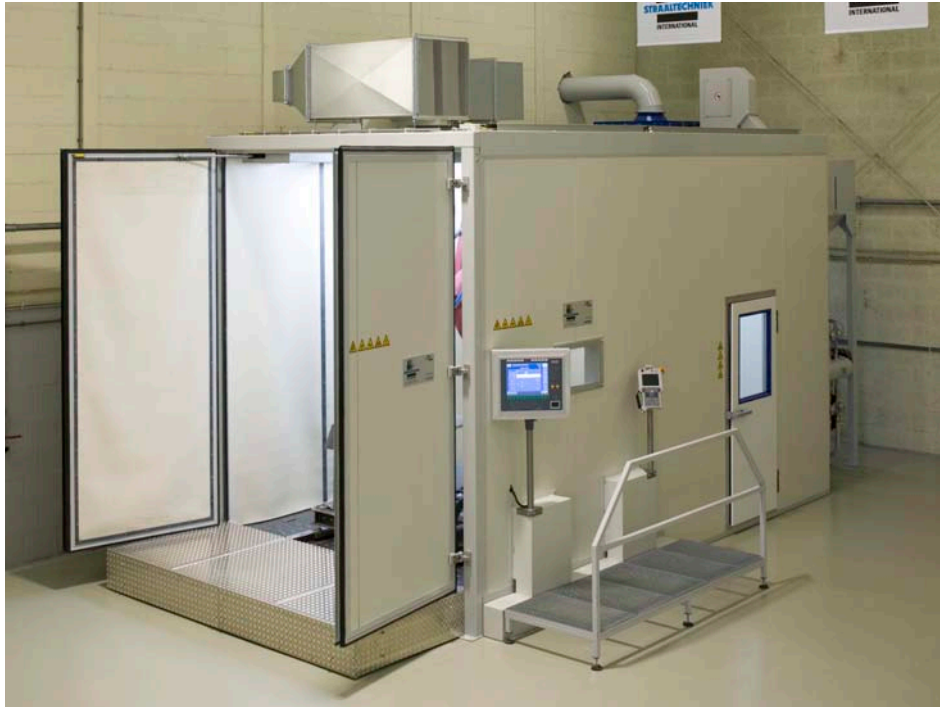
Robotic shotpeening machine with 10 NC-axis at Straaltechniek International, used as jobshotpeening in Holland
