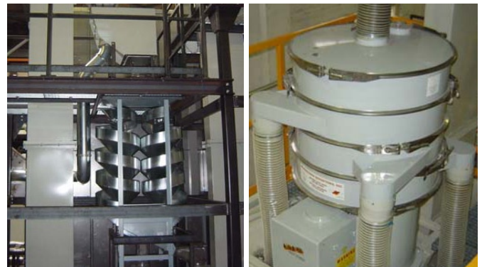
Elevator with spiral separator on the left image Medium size classifier on the right image
