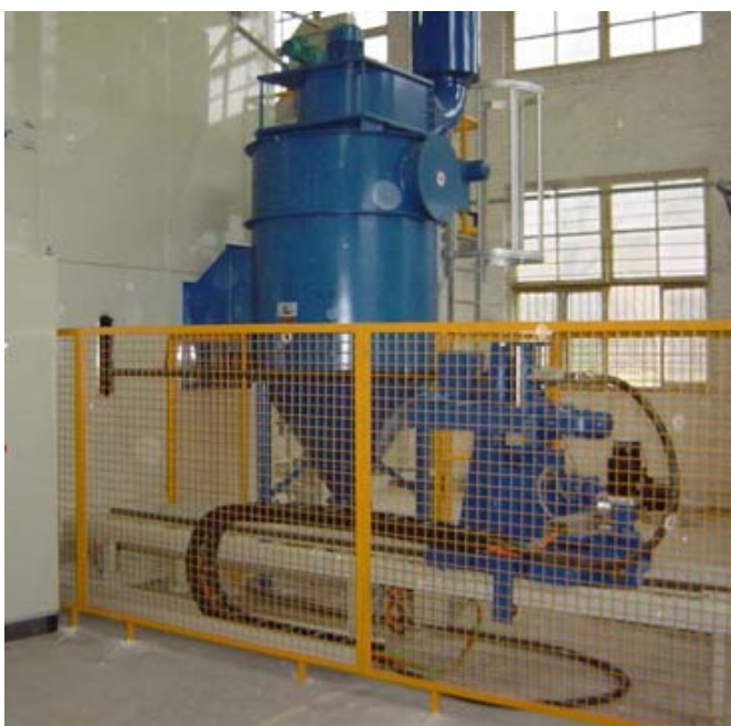
Horizontal lance for deep hole peening
