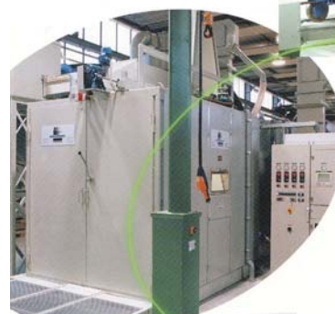
Shotpeen installation supplied to the Dutch Airforce is designed specially for all workshop repairs to cover a broad spectrum national requirements.
