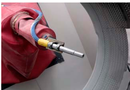
Internal- External blasting nozzle on robotic arm
