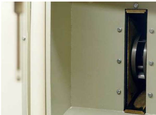
Turbine at the outside of the wheelpeening machine (top) and a view of the turbine from the inside of the wheelpeening machine.
